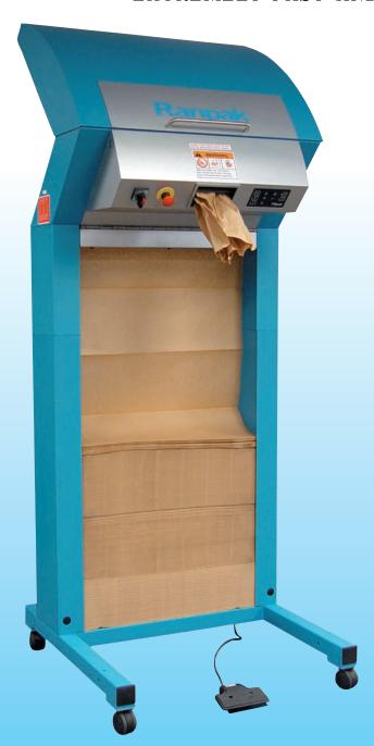
FillPak converts fanfold paper into a fast, efficient and effective voidfill material that will protect your products during shipment.
